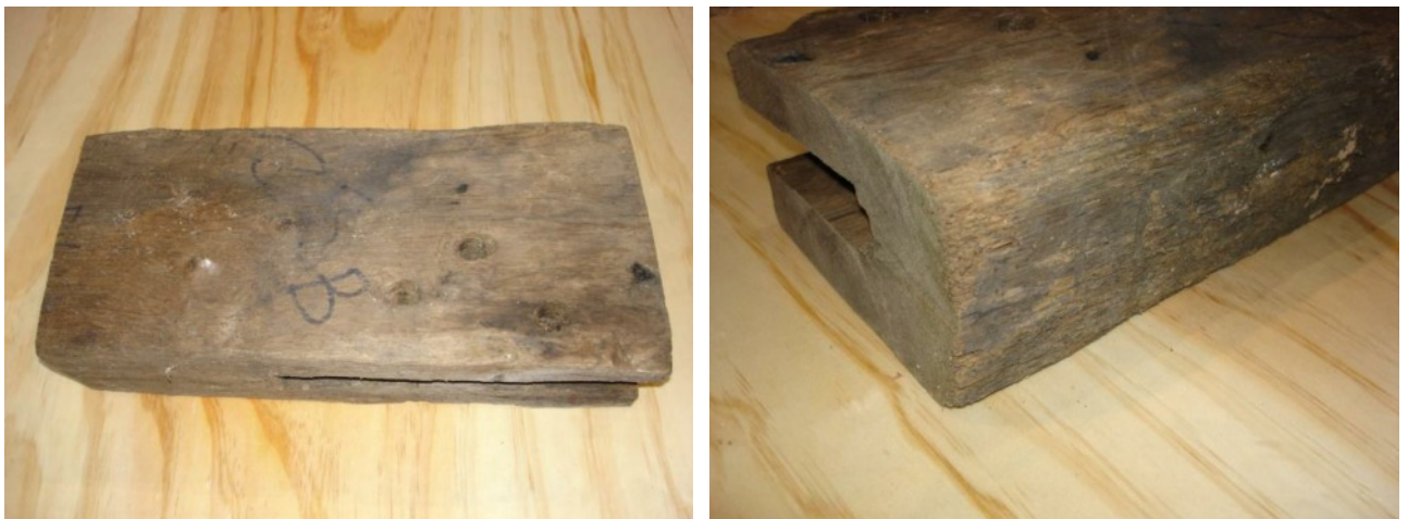
Fig 1b: Timber angg02 showing location of sample slice with III chiselled carpenters' mark
