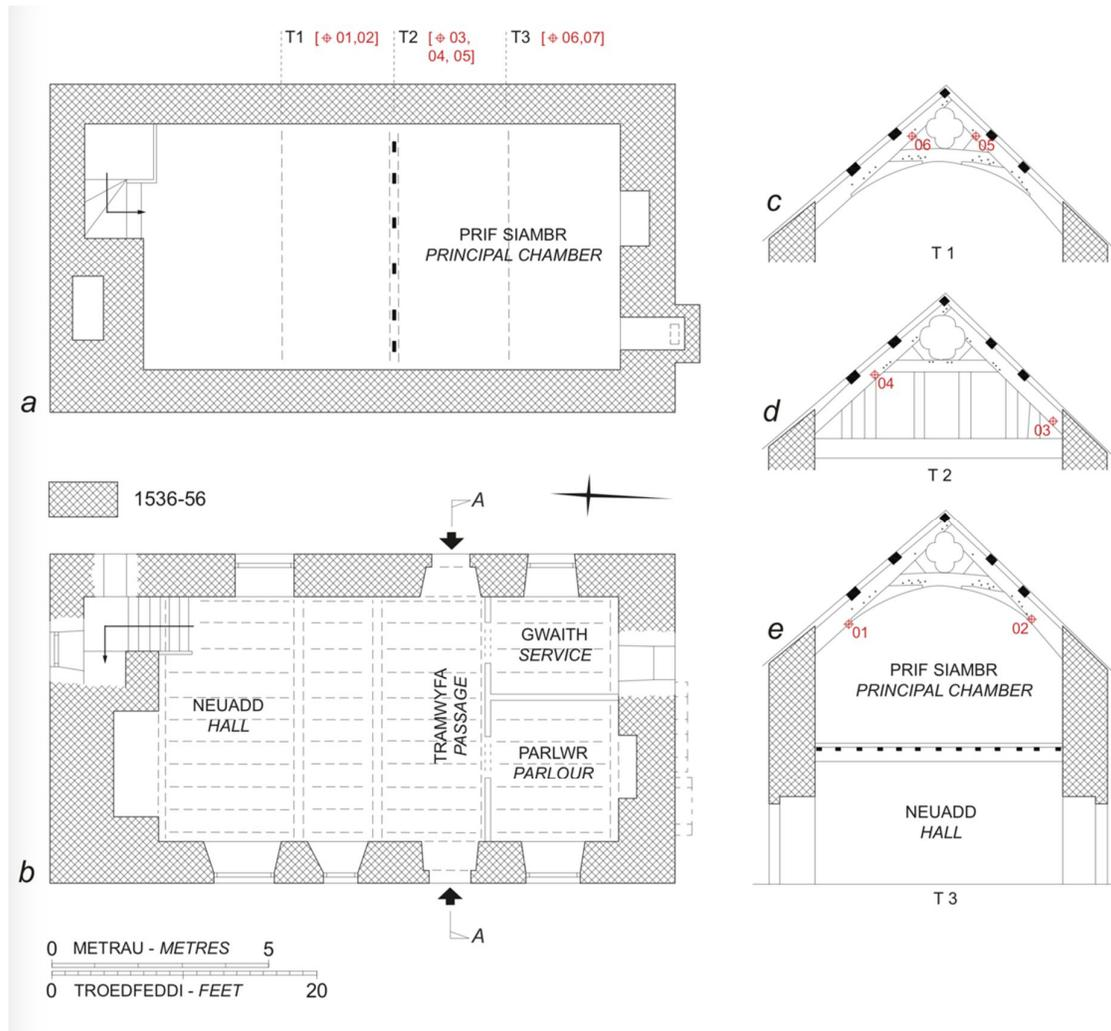
Above, plans (reconstructed) and sections (a) 1<sup>st</sup> floor; (b) ground floor; (c-e) trusses: the red numbers show the location of tree-ring samples. Dunn & Suggett, *Discovering the Historic Houses of Snowdonia*, 178. Crown Copyright: RCAHMW. The red figures indicate the location of tree-ring samples.
