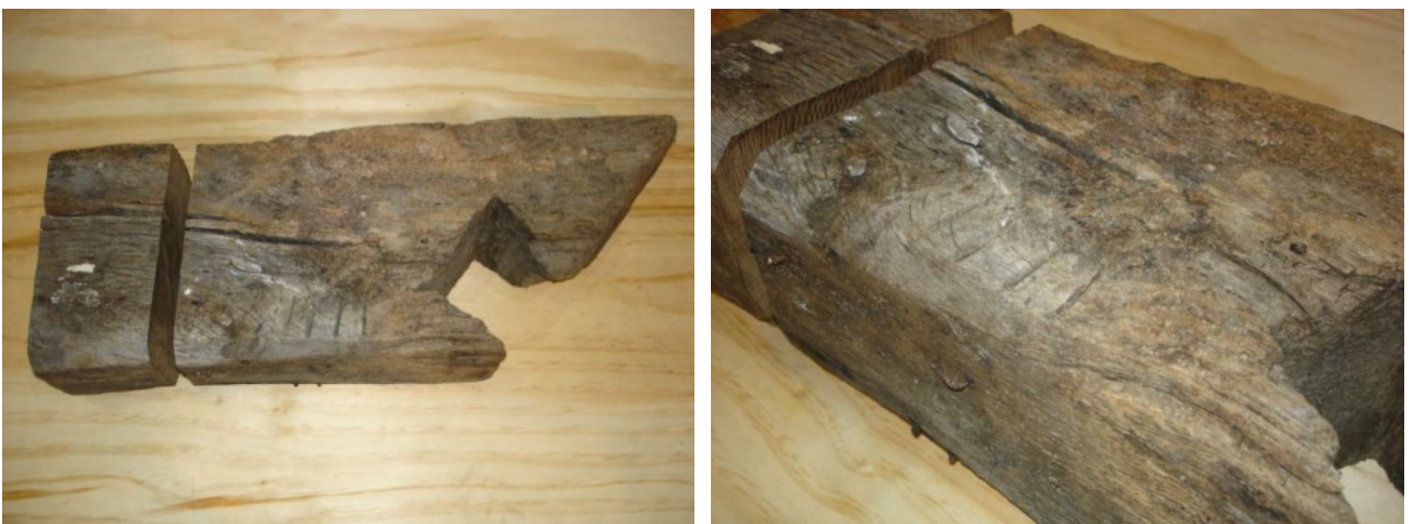
Fig 1e: Timber angg05 showing location of sample slice with IIII chiselled carpenters' mark
