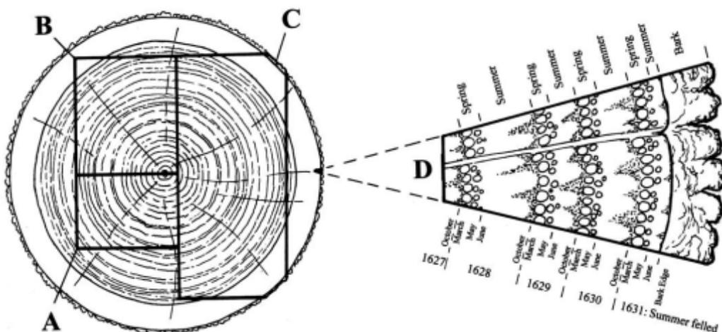
Section of tree with conversion methods showing three types of sapwood retention resulting in **A** *terminus post quem*, **B** a felling date range, and **C** a precise felling date. Enlarged area **D** shows the outermost rings of the sapwood with growing seasons (Miles 1997, 42)
