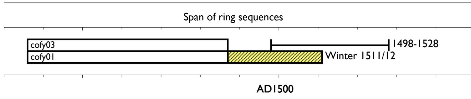
**Figure 1:** Bar diagram showing the relative positions of overlap of the dated samples, with their actual or likely felling dates / date ranges. White sections represent heartwood rings and yellow hatched sections represent sapwood.
