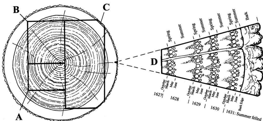
Section of tree with conversion methods showing three types of sapwood retention resulting in **A** *terminus post quem*, **B** a felling date range, and **C** a precise felling date. Enlarged area **D** shows the outermost rings of the sapwood with growing seasons (Miles 1997, 42)
