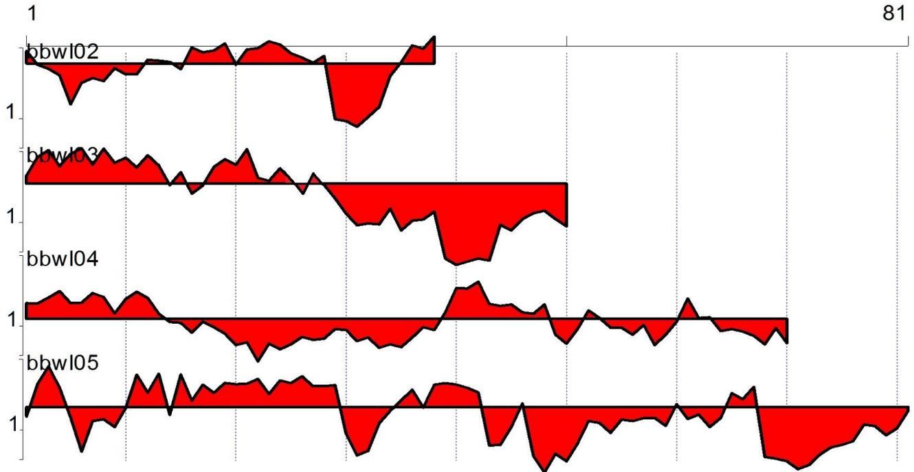
**Figure 2:** Plots of the roof samples showing the sudden growth rate changes in all but sample **04**. The y-axis is ring width (mm) on a logarithmic scale. The horizontal line through each plot denotes the mean ring width of the individual series.
