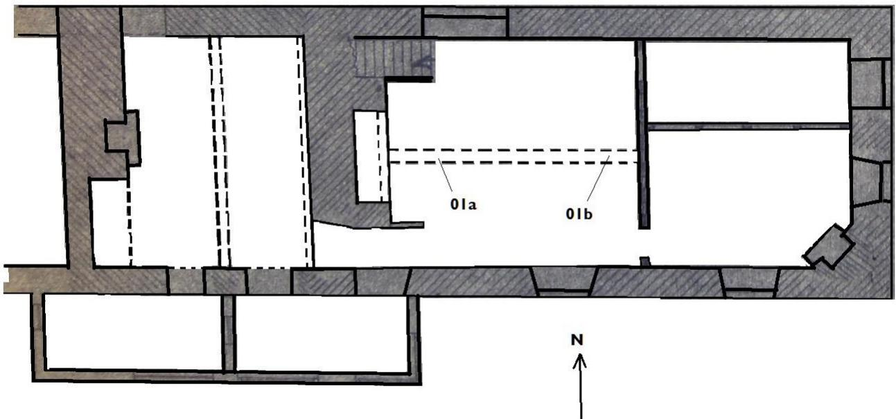
**Figure 1:** Ground floor plan showing the axial beam sampled in two places, adapted from an original drawing by Ffrangcon Lloyd
